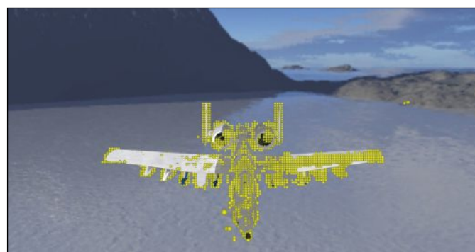
FIGURE 5 A point cloud sensed by the tanker's stereo cameras.
