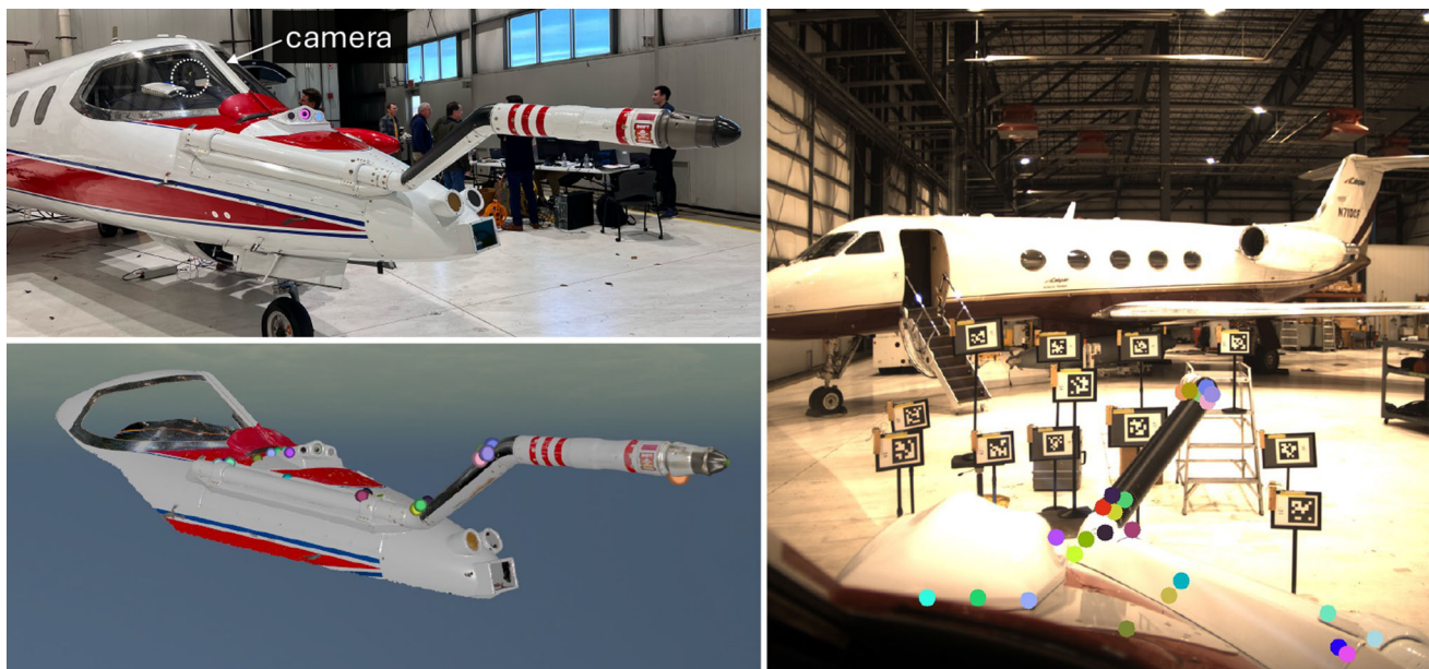
Fig. 17 The top left image depicts the Learjet 25 receiver aircraft retrofitted with a refueling probe and cockpit-mounted camera. The portion of its nose seen by the camera was 3D scanned (bottom left)
