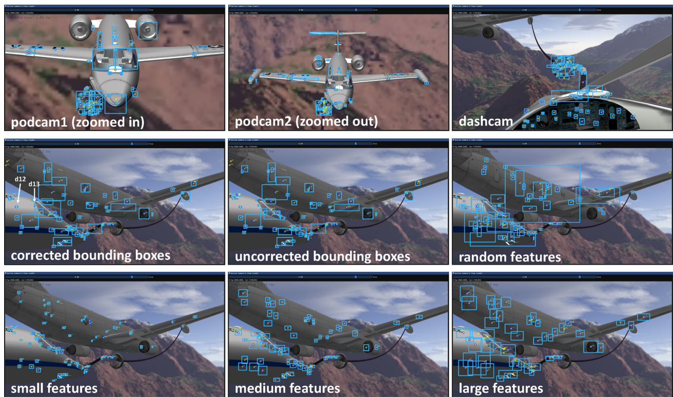
Fig. 13 Experimental vantage points. Light blue rectangles and dark blue circles depict YOLO predicted bounding boxes and corresponding bounding box center points, respectively, while the yellow circles depict true 2D feature points
