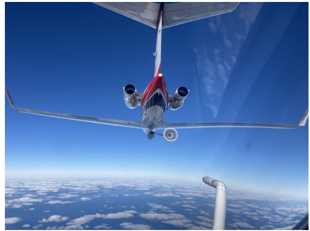
Fig. 1 The pilot must see both the probe and drogue during aerial refueling operations
