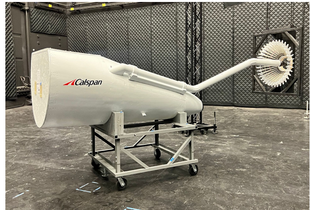
Fig. 30 Learjet nose cone and refueling drogue in a Vicon motion capture room
