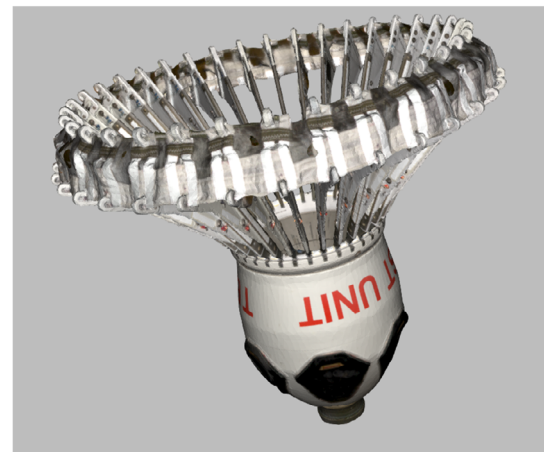
Figure 1. Artec Studio 17 Render of Drogue Model.
